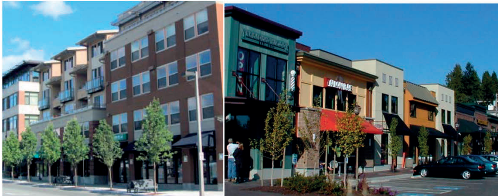
Figure 11 – Facade Examples Employing Building Walls with Contrasting Articulation That Make It Appear Like Two or More Distinct Buildings
