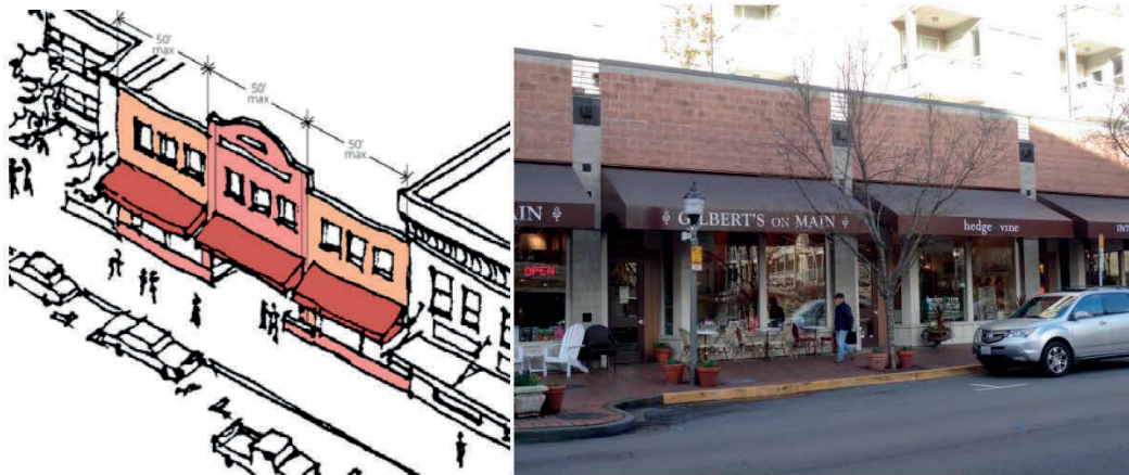
Figure 13 – Minor Facade Modulation Examples
